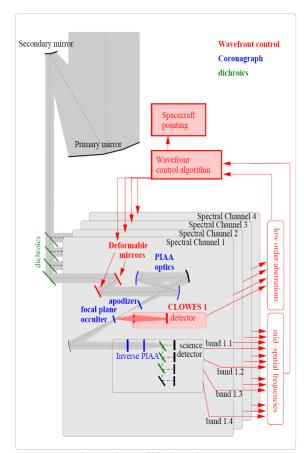
Figure 2. PECO Architecture
