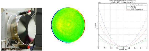
Figure 3. Left: a PIAA mirror, showing obvious asphericity. Center: Double-pass wavefront measurement of the aligned PIAA2 system at JPL's HCIT (color stretch is 1.8 waves). Right: Order-of-magnitude estimate of wavefront control performance for such a system. For this simulation, perfect correction was set at the central wavelength (800nm) and the degradation at other wavelengths was computed.
