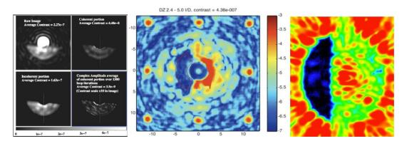
Figure 4. *Left*: Subaru testbed, 2e-7 contrast from 1.6-4  $\lambda$ /D, monochromatic light; *Center*: Ames testbed, 4e-7 contrast from 2.4-5  $\lambda$ /D, monochromatic light; *Right*: HCIT (BLC Coronagraph), 8e-10 contrast from 4-10  $\lambda$ /D in 10% band.
