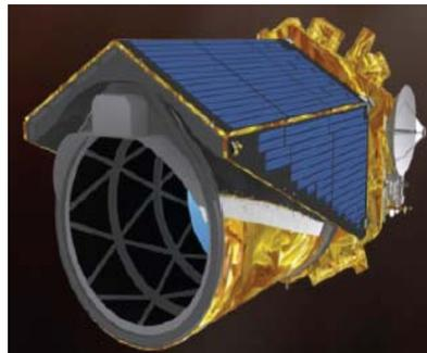
Figure 3: Concept payload for EPIC
