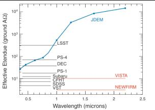
Fig 2. Effective etendue (product of field of view and telescope area, with corrections for sky brightness, duty cycle, and angular resolution) for JDEM and ground facilities. Horizontal lines show ground facilities. JDEM is a factor >300 faster than the ground at J, H, and K. Beyond the etendue statistic, space observations offer greater stability, guaranteed cadence, and the ability to resolve small galaxies. These advantages are critical for the weak lensing and supernovae programs.
