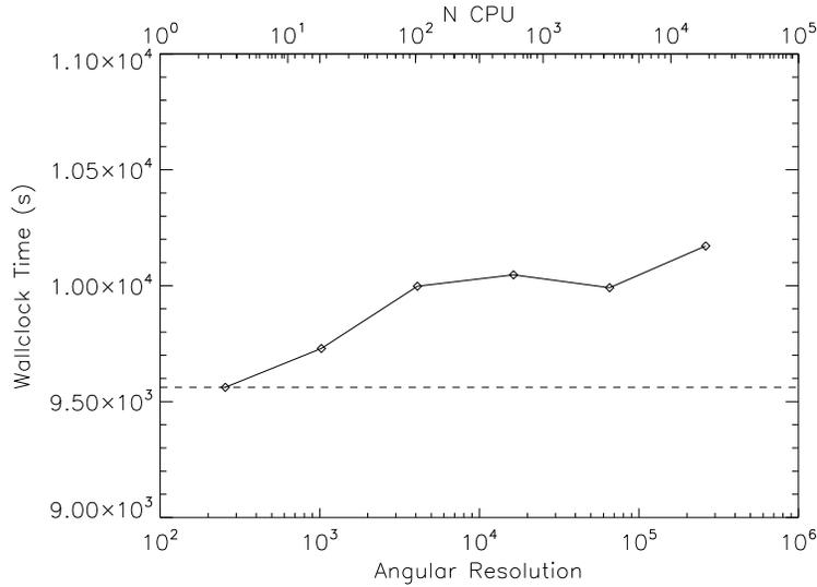
Fig. 2.— The wall-clock time to solve a scattering line  $\epsilon = 0.1$  on the the NERSC Franklin Cray-XT4 as a function of momentum frame angular resolution. The test was run so the amount of computational work per processor was constant. The dashed horizontal line indicates perfect scaling. The roughly 14% communication time increase from 16 to 16,384 processors is acceptable.
