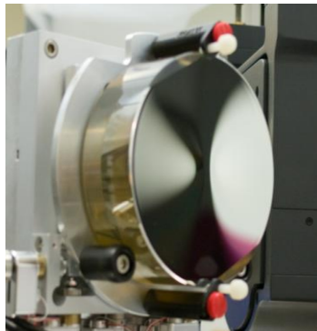
Figure 3. Left: a PIAA mirror, showing obvious asphericity. Center: Double-pass wavefront measurement of the aligned PIAA2 system at JPL’s HCIT (color stretch is 1.8 waves). Right: Order-of-magnitude estimate of wavefront control performance for such a system. For this simulation, perfect correction was set at the central wavelength (800nm) and the degradation at other wavelengths was computed.
