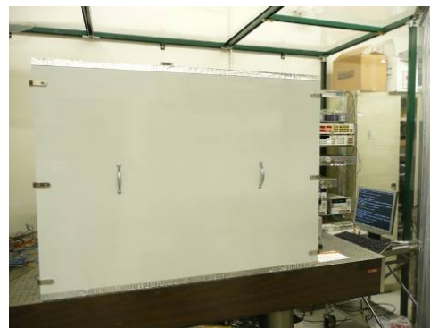
Figure 12. Newly constructed multi-layer thermal chamber.
