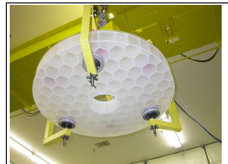
Figure 3: ITT's NextView 1.1m ULE ® frit PM is the heart of the Geo-Eye 1 Nextview Telescope
