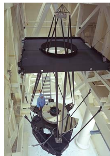
Figure 2: ITT started the development of segmented PMs in the 1980's
