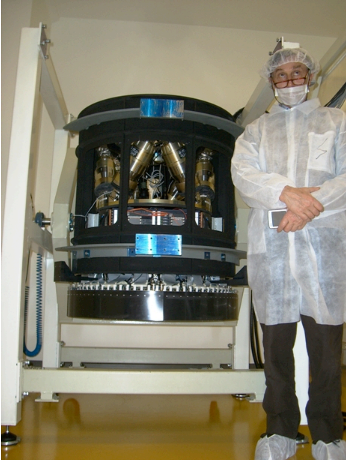
The first adaptive secondary mirror unit near completion of electromechanical acceptance.
