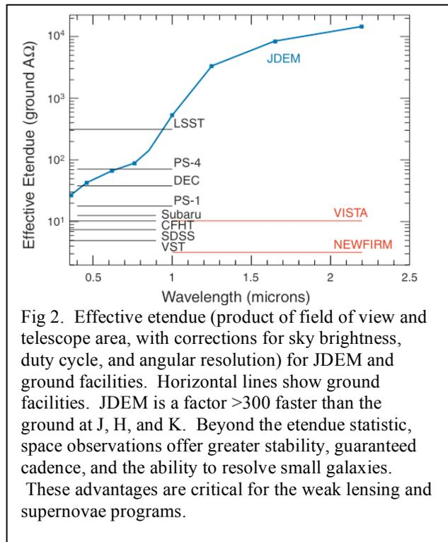
Fig 2. Effective etendue (product of field of view and telescope area, with corrections for sky brightness, duty cycle, and angular resolution) for JDEM and ground facilities. Horizontal lines show ground facilities. JDEM is a factor  $>300$  faster than the ground at J, H, and K. Beyond the etendue statistic, space observations offer greater stability, guaranteed cadence, and the ability to resolve small galaxies. These advantages are critical for the weak lensing and supernovae programs.
