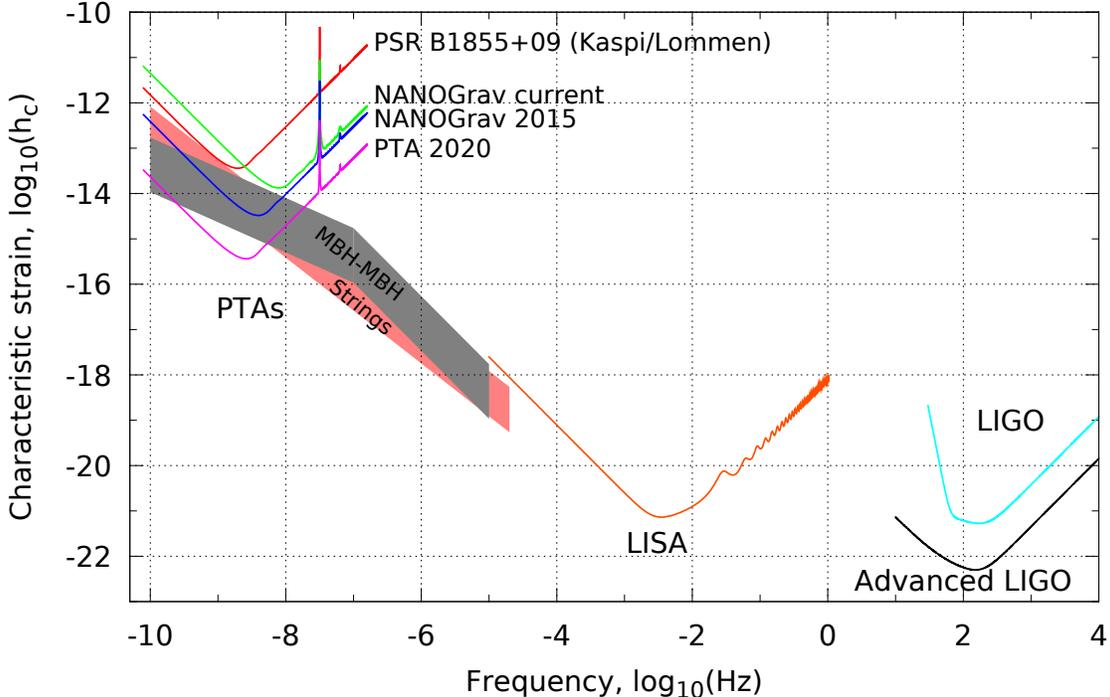
Figure 1: Comparison of current and planned GW detectors, showing characteristic strain ( $h_c$ ) sensitivity versus frequency along with expected source strengths. The Laser Interferometer Gravitational Wave Observatory (LIGO), the Laser Interferometer Space Antenna (LISA) and PTAs occupy complementary parts of the GW spectrum.
