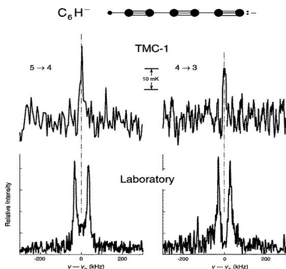
**Figure 2:** The interstellar detection of C<sub>6</sub>H<sup>-</sup>, showing astronomical data (upper) and the laboratory measurements (lower) that made the identification possible (McCarthy et al. 2006)
