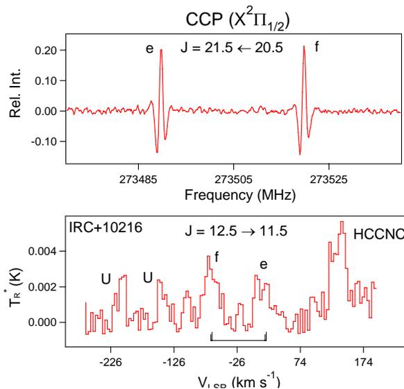
**Figure 3:** Detection of CCP in IRC+10216, showing laboratory (top) and astrophysical (bottom) spectra of CCP ( $X^2\Pi_r$ ); the lambda-doublets are labeled by e and f in each transition. The astronomical spectra were measured with the ARO 12 m telescope (Halfen et al. 2008)
