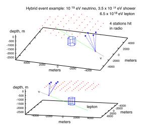
Figure 3: Simulation of an incident  $10^{19}$  eV neutrino which deposits 35% of its energy into a shower that was seen by 4 of the subsurface radio detectors (red dots), while the secondary lepton passes just outside the Ice-Cube array (blue hexagon) and is detected with an energy of  $6.5 \times 10^{18}$  eV.
