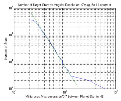
Number of target stars versus angular resolution of a coronagraph, for stars brighter than 7 magnitude and star planet contrast > 6e-11, for an Earth clone in mid-habitable zone.
