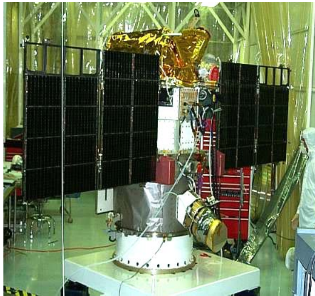
Figure 1. The DSCOVR spacecraft in a Goddard SFC clean room.
