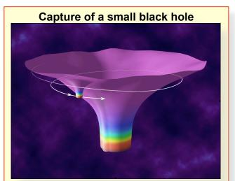
Figure 3: Embedding diagram of an EMRI, with the smaller black hole orbiting in the spacetime of the larger black hole. The colors depict the slowing of time (the "lapse" function) as one nears the horizons and the shape depicts the geometry of space in the orbital plane.
